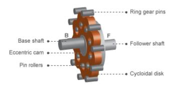
During normal operation, the base shaft drives the eccentric cam. The cam spins inside the cycloidal disk, causing it to rotate in an eccentric pattern about an offset axis. As it moves, the cycloidal disk engages the internal teeth of the ring-gear housing. The internal meshing reverses the rotational velocity direction.
