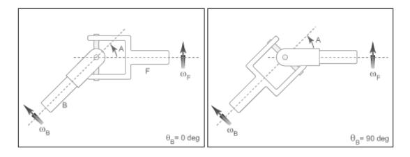
In the figure, the intersection angle is the angle between the two shafts about the base shaft's pin. The absolute value of this angle must fall in the range  $0 \le A < Maximum$  intersection angle. The base shaft angle is the angle of the base shaft about its length axis. The base shaft angle is also the time-integral of the base shaft angular velocity,  $\omega_B$ .
