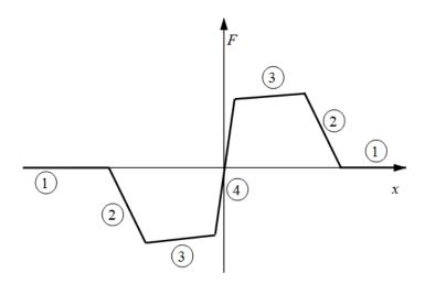
Because the ball is spherical and the notch is symmetric, the horizontal force versus displacement function is symmetric about the origin. (See "Peak Force and Notch Width" on page 1-346.)
