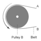
The block dialog box enables you to select the relative belt direction of motion. Depending on the chosen setting, the two belt ends can move in equal or opposite directions. The block model assumes noncompliance in the belt and no resistance to motion due to wrapping around the pulley.
