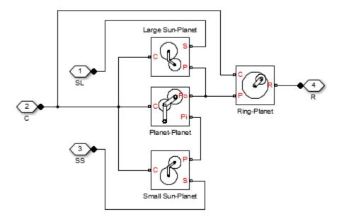
To increase the fidelity of the gear model, you can specify properties such as gear inertia, meshing losses, and viscous losses. By default, gear inertia and viscous losses are assumed negligible. The block enables you to specify the inertias of the internal planet gears only. To model the inertias of the carrier, large sun, small sun, and ring gears, connect Simscape Inertia blocks to ports C, SL, SS, and R.
