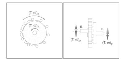
The cycloidal drive can operate in reverse mode, e.g., with power flowing from the follower shaft to the base shaft. In this mode, torque transfer efficiencies are typically negligible. You can adjust the efficiency value in the block dialog box using the **Efficiency from follower shaft to base shaft** parameter.
