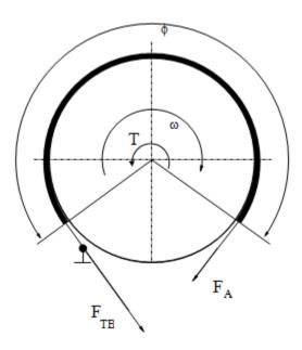
The following formula provides the braking torque as a function of the external brake actuation force that tightens the belt.
