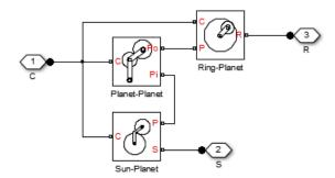
You can model the effects of heat flow and temperature change through an optional thermal conserving port. To expose the thermal port, right-click the block and select **Simscape > Block choices > Show thermal port**. Exposing the thermal port causes new parameters specific to thermal modeling to appear in the block dialog box.
