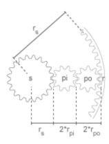
In terms of the ring-sun and outer planet-inner planet teeth ratios, the ring-outer planet teeth ratio is
